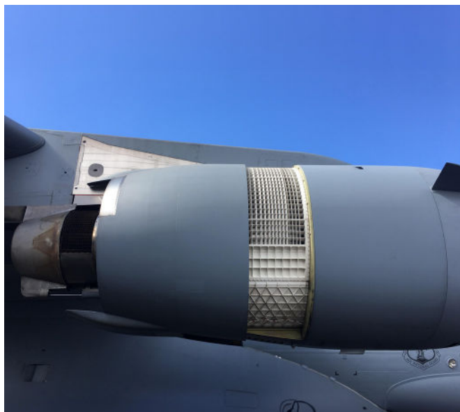
Figure 3. C-17 wing mounted F117 nacelle with thrust reverser deployed, showing cascades for providing reverse flow on upper half of the nacelle only.
