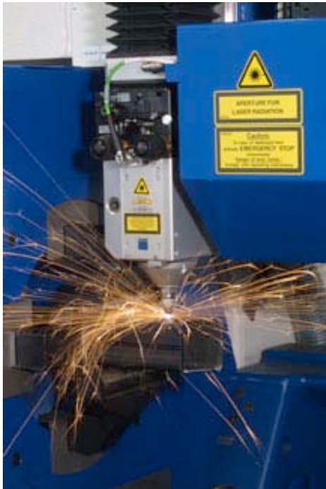
The TRUMPF TUBEMATIC™ uses a laser to accurately and precisely cut metal tubes and pipes. (Photo courtesy TRUMPF Inc.)
