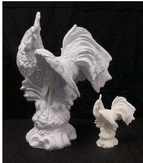
At Bolton Works in East Hartford, a plaster rooster garden sculpture, left, was purchased online and 3D scanned. The scanned data was then printed on one of the company's 3D printers. The 3D printed version is on the right. [Photo: Bolton Works]
