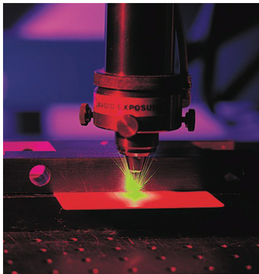
Ceramic scribing with a Coherent Diamond K250 CO 2 Laser. [Photo courtesy of Coherent]
